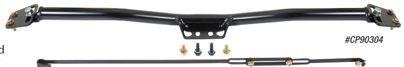
CHEVELLE CROSSMEMBERS SHOWN WITH PARKING BRAKE CABLE BRACKETS
