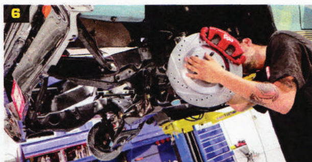
On Day 2, we dove into the Chevelle's suspension installation. The CPP spindles utilized modern Corvette sealed bearings so it was nice not having to mess with packing wheel bearings with grease. It also saved us a lot of time. To help move things along CPP sent over a few of their technicians.
