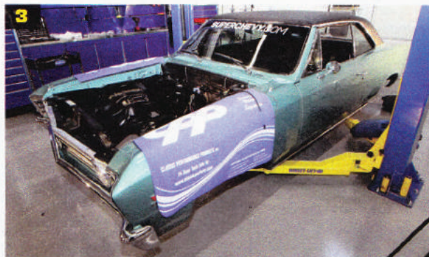
After four hours we had removed the drivetrain, suspension, brakes, rearend, and most of the wiring. By lunch on the first day, we were feeling pretty confident.
