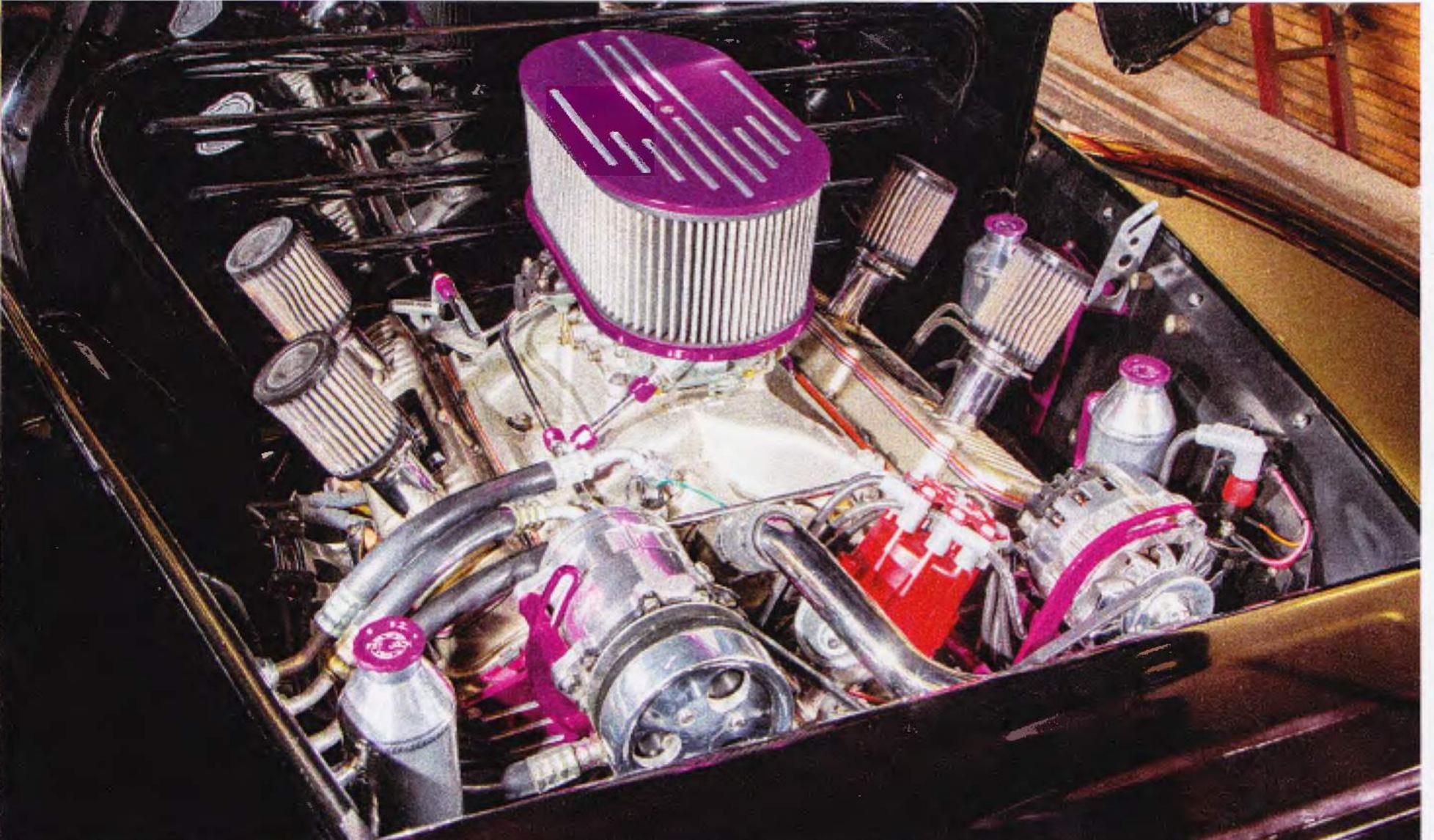
[With the plumbing and breathers, it's hard to tell this is a 1967 430 Buick punched out to 444 ci, built by Jack's son, John. Firewall, fender panels, and core support were all fabbed at Fat Jack's.
