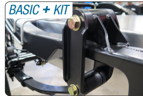
BASIC + KIT LEAF SPRING POCKET INSTALLED
